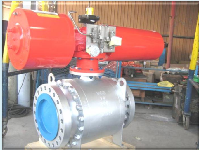
A UCM ball valve has been adopted by PETRONAS Carigali Sdn as a shut down valve CL600 – 14" Forged Steel Ball Valve with Bettis actuator
