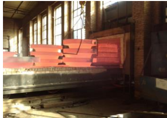
ASTM A694 F70 FLANGE 28" 600LBS WN RF SCH.14.28MM ASME B16.47 SERIE A HEAT TREATMENT AND QUENCHING
