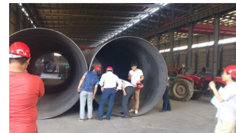
SPIRAL WELDED PIPE 2400MM
