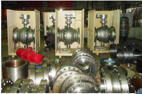
20" x ANSI 150LBS 316SS TRUNNION & SMALL CARBON STEEL BALL VALVE FOR POLYACETAL PLANT IN THAILAND
