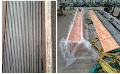
SS SMLS TUBE A269, A213 & WOODEN CASE PACKAGE
