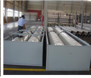
SS WELDED PIPE A312 24" & STEEL CRATE PACKAGE
