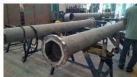
316L FLANGE, FITTING, SMLS PIPE
